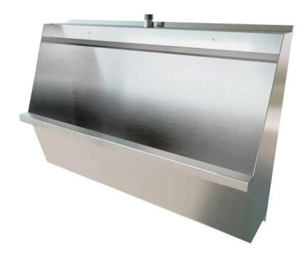
Our budget wall hung urinal style is fabricated from single piece 304 grade stainless steel in an attractive and durable design. The wall hung style offers the advantages of easy installation and maintenance. Perfect for temporary or transportable facilities and ablution blocks. Inbuilt fixings allow unit to be fastened directly to wall without requirement for brackets. Comes supplied with removable domed outlet grate. WELS and WaterMark certified.
