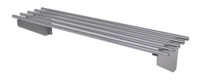
The Simcraft Tubular Shelf is hand-crafted from 1.2mm thick 304 grade stainless steel. The shelves manufactured to 4 standard sizes, however custom size can be manufactured on request. Each shelf is 300mm wide and supplied with stainless steel wall brackets. A cost effective storage solution idea for canteens, commercial kitchens and restaurants
