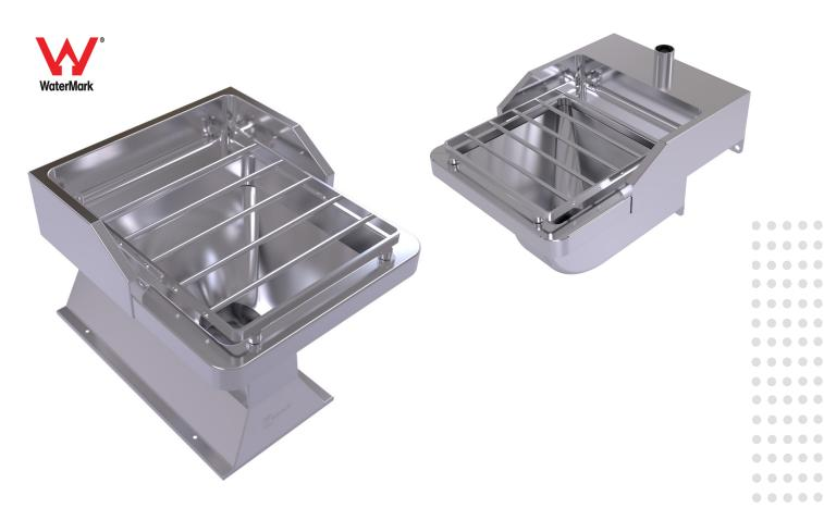
The Simcraft Slop Hopper is a heavy duty unit designed for quick, efficient and hygienic disposal of waste. The unit is hand-crafted from 316 grade stainless steel, and features a flushable bowl design and in-built P-trap or S-trap allowing for immediate removal of any waste placed into the unit. The unit features a removable hinged grate for support and storage, and can be manufactured in floor-mounted or wall-hung configurations. Ideal for medical facilities or laboratories.
