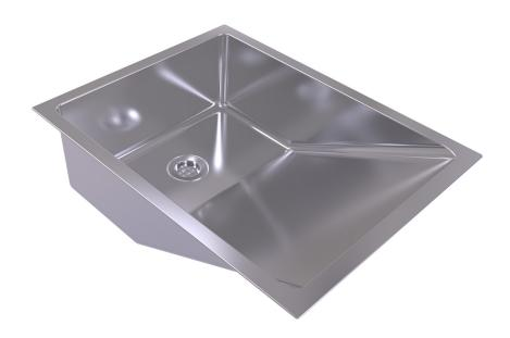
The Simcraft Baby Bath Basin is crafted from 304 grade stainless steel, and features a gentle gradient at the front side to facilitate easy and comfortable bathing of infants. The unit is manufactured with radius internal corners for efficient and complete cleaning, and can be supplied with pre-plumbed tapware and/or extended rear hob. This unit can be configured as inset, wall hung or free-standing, and is supplied as standard with WaterMark certified 50mm plug and waste.
