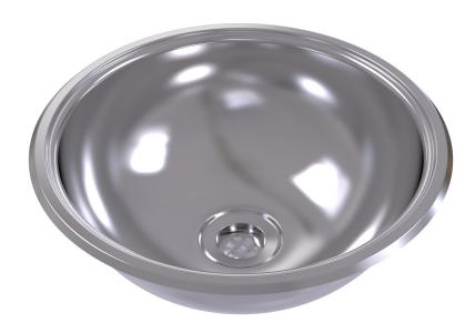
The Simcraft Round Bowl Basin is an economical and attractive solution suitable for a wide range of applications. The unit is fully pressed from 304 stainless for a seamless surface, and has a bright finish for easy cleaning. This basin is supplied in a standard size, and comes with inset clips and WaterMark certified 50mm waste.
