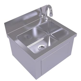
The Simcraft Knee Operated Basin is a heavy duty wall-mounted unit perfect for use in ablutions by multiple users where cross-contamination may be an issue. The unit is made in 304 grade stainless steel as standard, and comes preplumbed with a tap fitted with tempering and time-flow valve, which is activated by pressing in the knee panel fitted to the front fascia of the basin. Also included are heavy duty wall brackets and WaterMark certified 40mm waste outlet.
