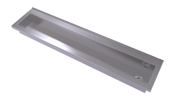
The Challenger Trough is an economical yet durable and versatile unit which is available in a range of standard sizes. Crafted from single sheet 304 stainless steel, the design features a 100mm rear hob for mounting tapware and rear tile lip for effective waterproofing. A blade upstand can be incorporated for additional splash protection on the surrounding area. Includes 50mm stainless steel outlet and heavy duty brackets for wall mounting.
