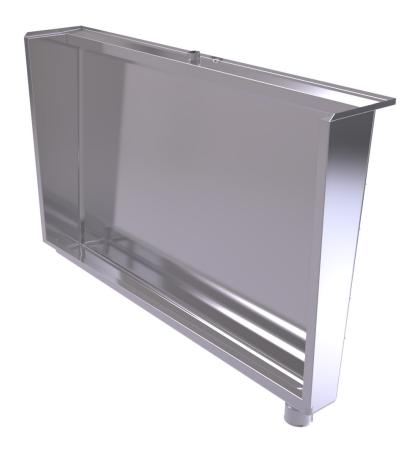
An economical, durable and easy to clean model, with a one piece design from 304 grade stainless and rear wall reinforcement providing decades of strength. Perfect for installation in confined areas or those with tile step or sloping/graded floors. Full-length flushing sparge ensures complete coverage of rear wall. Comes supplied with removable domed outlet grate. WELS and WaterMark certified.
